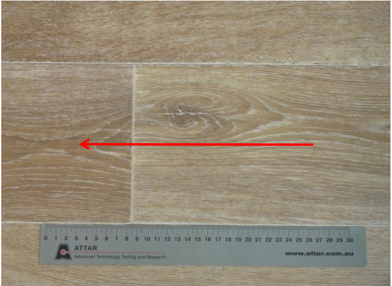
Figure 1: Taralay Impression Compact with ProtecSol sheet vinyl Arrow indicates direction of testing
